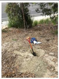
Photo 6: View of Sample Pit 4. Note dry, sandy (non-hydric) soils. Lacks vegetation and hydrology.
