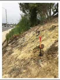
Photo 4: View of Sample Pit 2. Note saturated soils and unvegetated conditions on slope next to Sample Pit 2. Cattails in distance.
